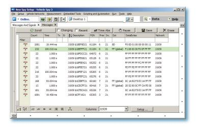
Vehicle Spy is used (and required) to configure stand-alone mode. Users can take advantage of the powerful interface to load databases and to write and debug scripts before downloading them to the device.
